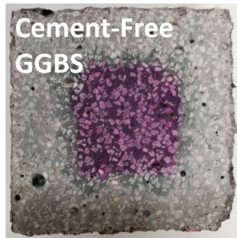
Accelerated carbonation tests (10% CO 2 )
