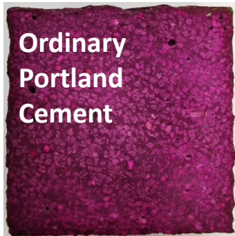
Accelerated carbonation tests (10% CO 2 )
